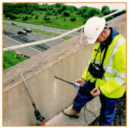
Elcometer Borehole Probe / Tendon Duct Locator
