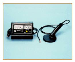
Elcometer P120 Rebar Locator
